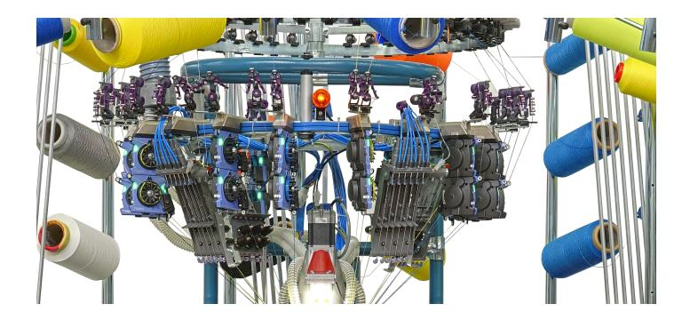
Single-cylinder INTARSIA electronic knitting machine with 4 reciprocating feeds and 2 selection points (3 technical ways) per feed and per rotating sense for the production of intarsia products with breathable mesh areas with cushioning and/or transfer stitch areas knitted in sculpted terry.
